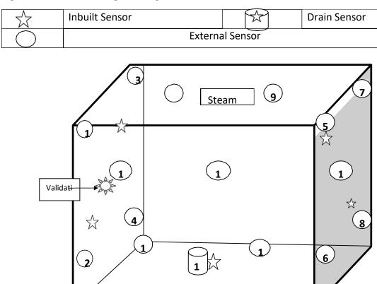
Set Parameters for Empty Chamber Heat Distribution Studies (HPHV Process) are as follows:
